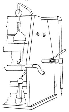
the tank and each is provided with a rubber tube to which a Hopkins<sup>11</sup> safety distilling bulb is attached.
